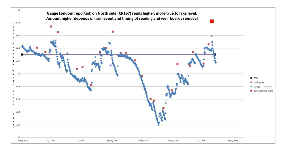
Data/measurements show how the gauge at the weir structure does not show true lake level. Region very near the weir drains quickly- difference in gauge transient readings note quick drop when level control boards were removed(\*) Subsequent timely close following storms would build on this difference
