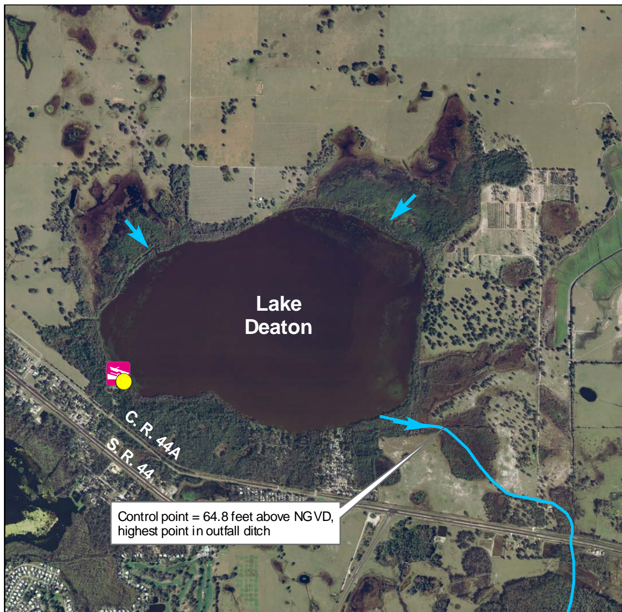
Figure 2. Location of lake water level gauge, public boat ramp, hydrologic indicators, inlets, outlet, outlet conveyance system, water control structure, and control point for Lake Deaton.
